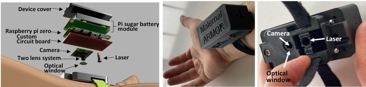
Figure 2. CAD rendering and photos of wearable SPG prototype that was designed and built.
