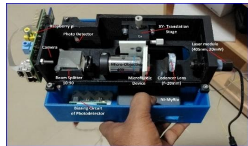
Figure 2: Developed Lab type prototype for same analysis using simple source, microfluidic device and simple electronics for malaria diagnosis at Point-of-Care (27)
