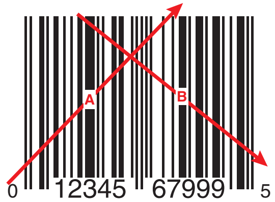
▲ Fig. 6. Simple X configuration scanning pattern.
