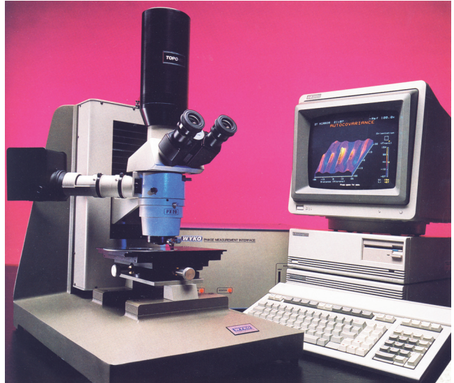
▲ Fig. 3. Phase-shifting interference microscope for measuring surface microstructure (1985).
