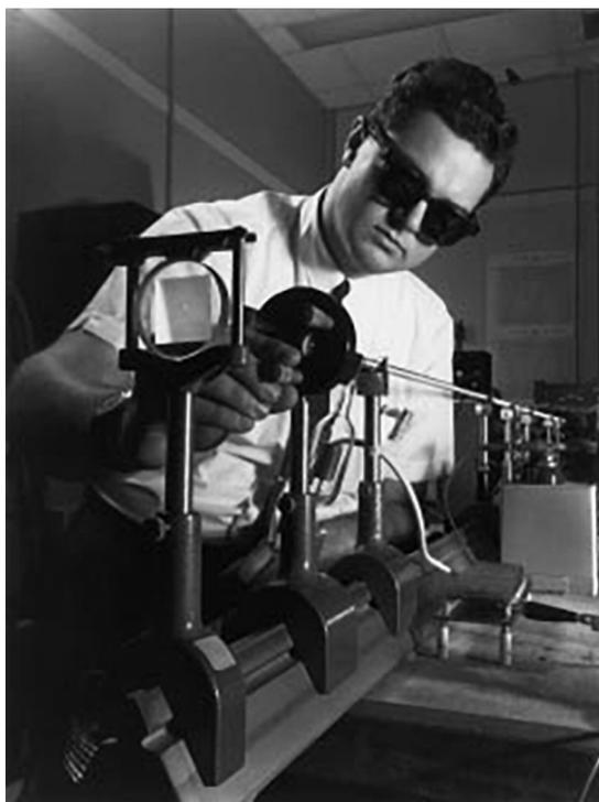
▲ Fig. 6. Photograph of the author with a pulsed argon-ion laser in his laboratory in February 1964: an air-cooled fused silica discharge tube with Brewster’s angle windows and external mirrors. Pulse lengths of a few microseconds with a simple capacitor discharge and rates of a few hundred per second were used.
