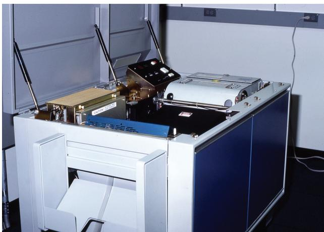
▲ Fig. 2. Dover printer with covers open.
