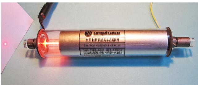
▲ Fig. 4. A simple helium–neon gas laser typical of those in supermarket optical scanners. The cavity mirrors are attached directly to the ends of the small diameter discharge tube. An aluminum cold cathode surrounds the discharge tube. Tubes like this sold for about \$100, and typically lasted for over 10,000 hours.
