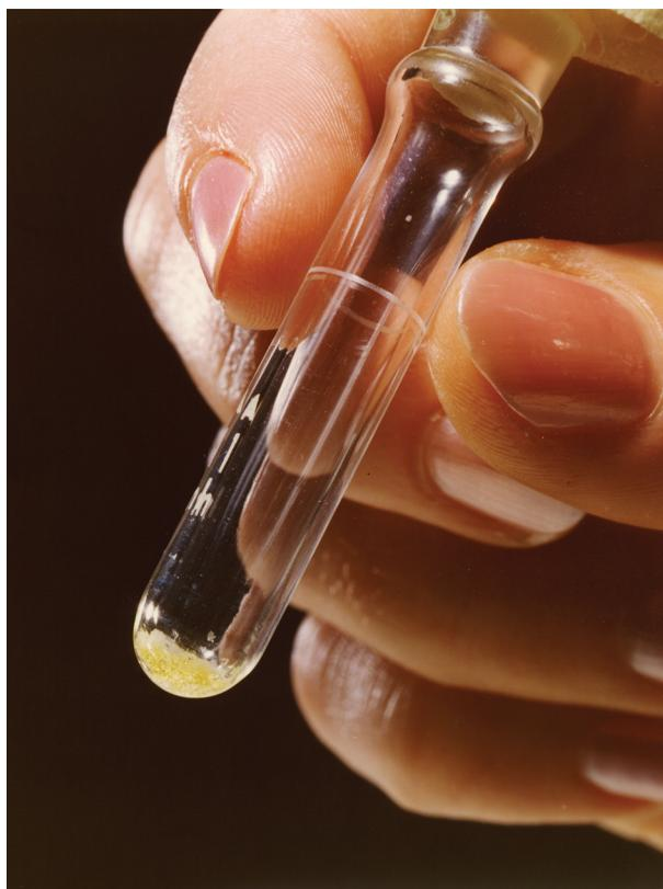
▲ **Fig. 2.** Four milligrams of uranium with its U-235 concentration enriched to 3% by a dye laser process at Livermore is visible at the bottom of this test tube—the first time this much uranium was enriched by lasers. 1975 photo from the Lawrence Livermore National Laboratory. (Lawrence Livermore National Laboratory.)
