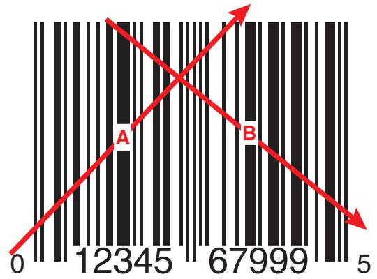
▲ Fig. 6. Simple X configuration scanning pattern.
