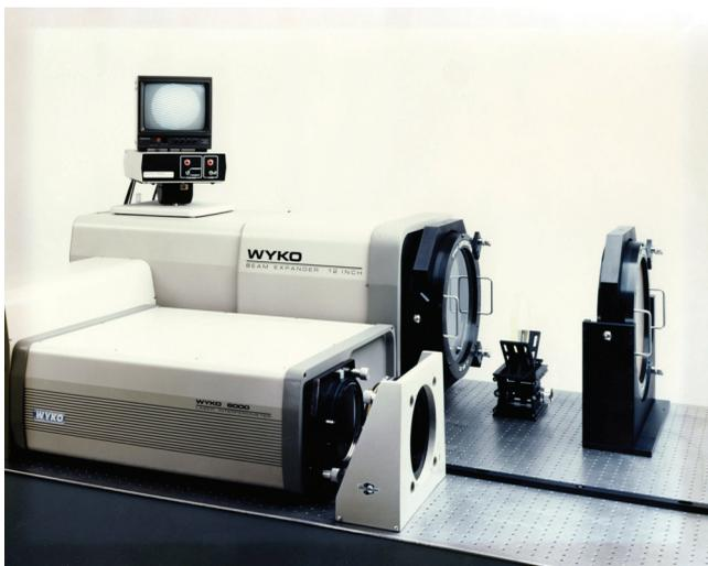
▲ Fig. 2. Laser-based phase-shifting Fizeau interferometer having both a 6-in. and a 12-in. aperture (late 1980s).
