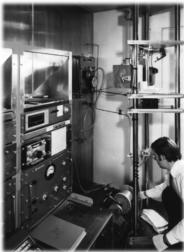
▲ Fig. 2. Clive Day working with his three-legged drawing tower at the Post Office Research Laboratories in Martlesham (UK) in the 1970s. (Courtesy Dr. Clive Day and the Post Office Research Centre, Martlesham Heath, UK.)
