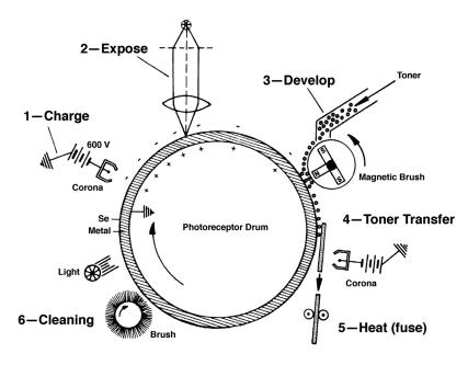
Fig. 4. The automated xerographic process using the six-step process. In brief, the original is scanned and projected synchronously onto a charged rotating photoreceptor drum. A toner development station develops the image on the photoreceptor and the copy paper is fed to transfer the image from the photoreceptor. The image is detached from the photoreceptor and then passed through toner fuser rolls.
