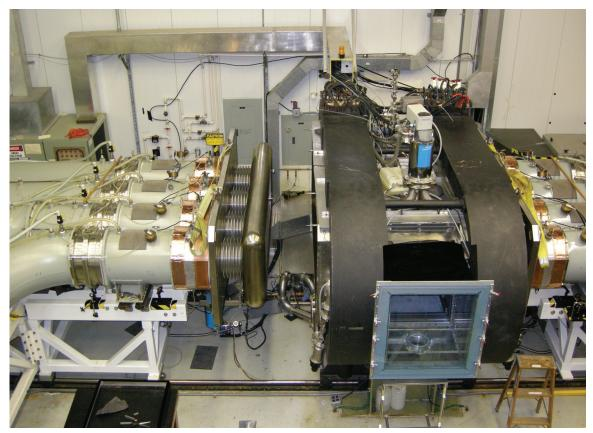
**Fig. 3.** The 60-cm aperture final amplifier of the Nike KrF laser. The amplifier is pumped from two sides by electron beams generated by the cylindrical pulse-forming lines. (Courtesy of Naval Research Laboratory.)
