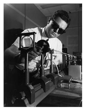
▲ Fig. 6. Photograph of the author with a pulsed argon-ion laser in his laboratory in February 1964: an air-cooled fused silica discharge tube with Brewster's angle windows and external mirrors. Pulse lengths of a few microseconds with a simple capacitor discharge and rates of a few hundred per second were used.
