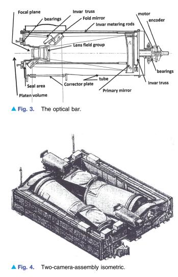
last lens. One optical bar was tilted 10 deg to look forward, and the other 10 deg to look back, creating a 20-degree stereo angle. A two-camera-assembly isometric is shown in Fig. 4.
