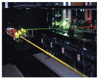
▲ Fig. 1. The Avco-Everett scheme for laser enrichment of uranium required the combination of four laser beams to produce the desired wavelengths to select U-235. (AVCO Research Laboratory, courtesy AIP Emilio Segre Visual Archives, Physics Today Collection.)
