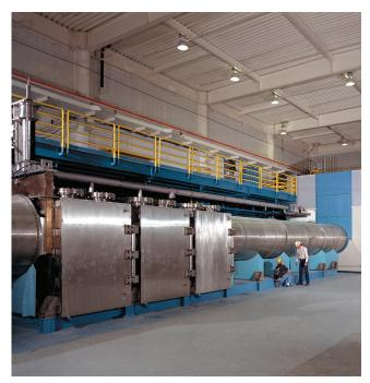
▲ Fig. 5. One of three units for separation of U-235 in Livermore's pilot plant for laser isotope separation. (Lawrence Livermore National Laboratory.)
