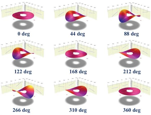
Fig. 4. Three-dimension contour maps showing shape of vibrating surface as a function of time.
