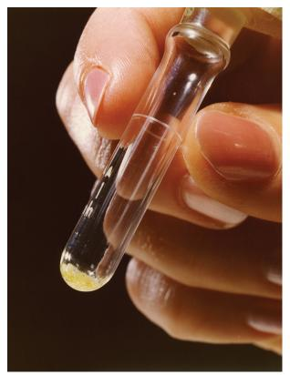
▲ Fig. 2. Four milligrams of uranium with its U-235 concentration enriched to 3% by a dye laser process at Livermore is visible at the bottom of this test tube—the first time this much uranium was enriched by lasers. 1975 photo from the Lawrence Livermore National Laboratory. (Lawrence Livermore National Laboratory.)
