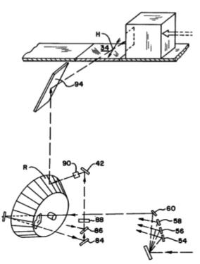
**Fig. 7.** A portion of the optical path in the Spectra-Physics scanner.
