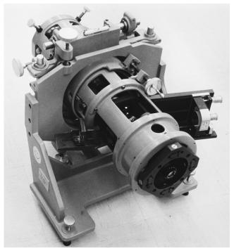
▲ Fig. 1. Laser unequal path Twyman–Green interferometer, often called a LUPI (1970).
