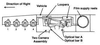
Fig. 2. Schematic of the entire Hexagon vehicle.
