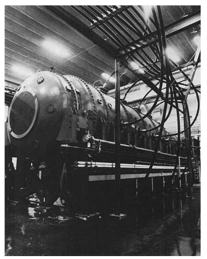
Fig. 2. Final amplifier of the Antares CO<sub>2</sub> laser system.
