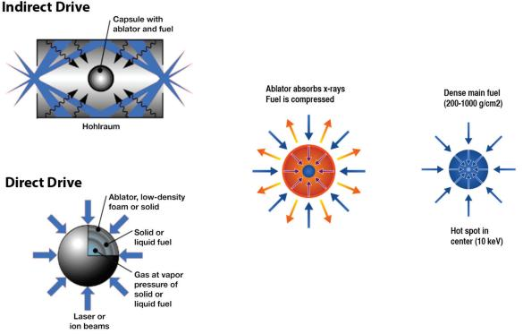
**Fig. 1.** In a direct-drive target, laser beams illuminate a fuel capsule uniformly. In an indirect-drive target, they illuminate the inside of a heavy metal hohlraum surrounding the target and are converted to soft x-rays. The x-rays then implode the fuel capsule.
