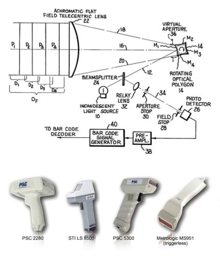
Fig. 8. Concept of U.S. patent 4,560,862: A rotating polygon with concave mirrors scans an image of an incandescent source across a barcode symbol.
