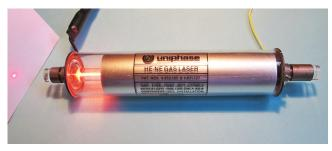
▲ Fig. 4. A simple helium-neon gas laser typical of those in supermarket optical scanners. The cavity mirrors are attached directly to the ends of the small diameter discharge tube. An aluminum cold cathode surrounds the discharge tube. Tubes like this sold for about \$100, and typically lasted for over 10,000 hours.
