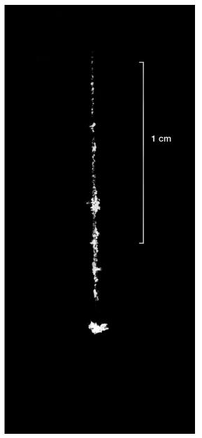
▲ Fig. 3. Trace of damage caused by a Q-switched ruby laser pulse. (Courtesy of Courtesy of Michael Hercher.)
