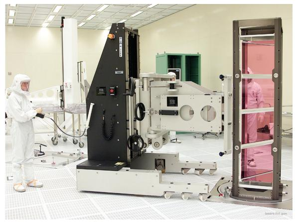
▲ Fig. 6. A stack of four NIF slabs ready for insertion into the final amplifier. (Courtesy of Lawrence Livermore National Laboratory.)
