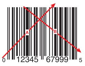
Fig. 6. Simple X configuration scanning pattern.
