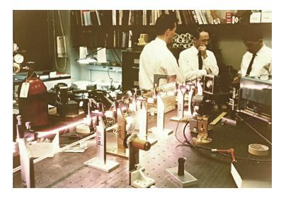
▶ Fig. 2. J. D. Rigden, A. D. White, and W. W. Rigrod with the first red He–Ne laser at Bell Laboratories. (Courtesy of Alan White.)
