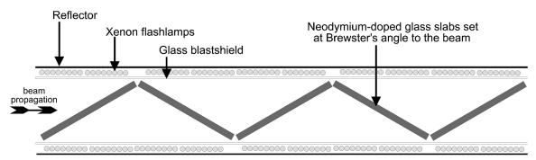
▲ Fig. 4. A Brewster's angle slab amplifier using neodymium glass. The laser beam sees no loss if it propagates through this series of slabs with polarization in the plane of the figure. (Courtesy of Lawrence Livermore National Laboratory.)
