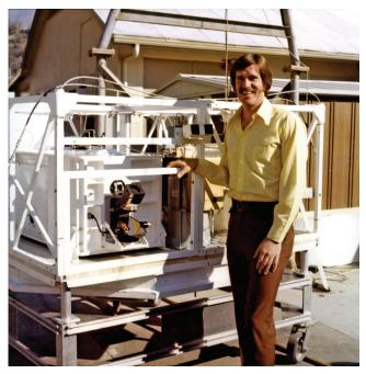
▲ Fig. 3. Photo of Bob Menzies and JPL laser heterodyne radiometer balloon instrument sitting in its gondola frame in 1979. (Courtesy of R. Menzies, JPL.)
