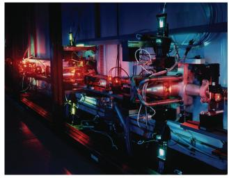
▲ Fig. 4. Copper-vapor pumped dye lasers scaled for uranium enrichment at Livermore. Most of the green light from the copper lasers was tightly confined so it could efficiently pump dye lasers, which emitted red-orange light tuned to three absorption lines of U-235 vapor. (Lawrence Livermore National Laboratory.)
