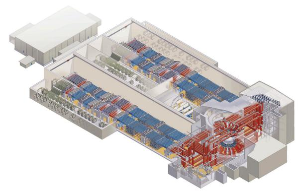
**Fig. 5.** The NIF laser fusion facility. NIF has 192 laser beams of 40-cm aperture and a 10-m diameter target chamber seen at the right end of the picture. (Courtesy of Lawrence Livermore National Laboratory.)
