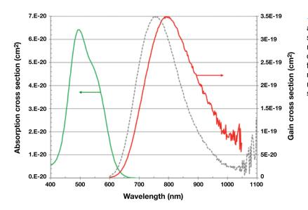
Fig. 2. Absorption (green) and emission (red) cross sections for Ti:sapphire and a relative plot (dashed gray curve) of the measured fluorescence spectrum. The noise in the long-wavelength region is from the detection system.
