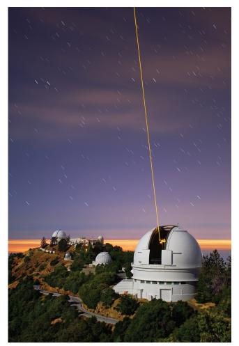
▲ Fig. 5. A laser guide star tuned to the wavelength of sodium atoms in the atmosphere, providing information on atmospheric turbulence to allow for adaptive optics to compensate and enable improved telescope resolution. (©Laurie Hatch.)
