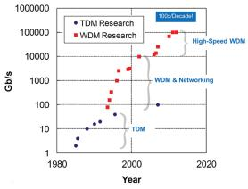
▲ Fig. 1. Reported research transmission systems experiments showing maximum transmission capacity over a single fiber vs. the year of the research results.
