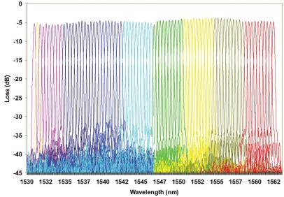
previously available. As multiplexing devices and amplifier performance was improved, the number of wavelengths was soon doubled and then quadrupled. In the research lab, work focused on WDM for higher TDM rates, 10 Gb/s and beyond.
