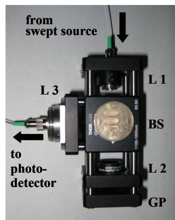
Fig. 2. Photograph of the common-path interferometer.
