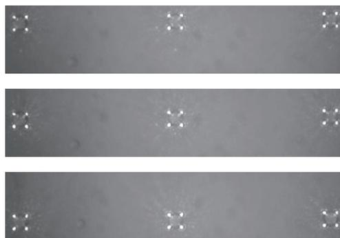
Fig. 5. Simultaneous transportation of three microdroplets at three positions.
