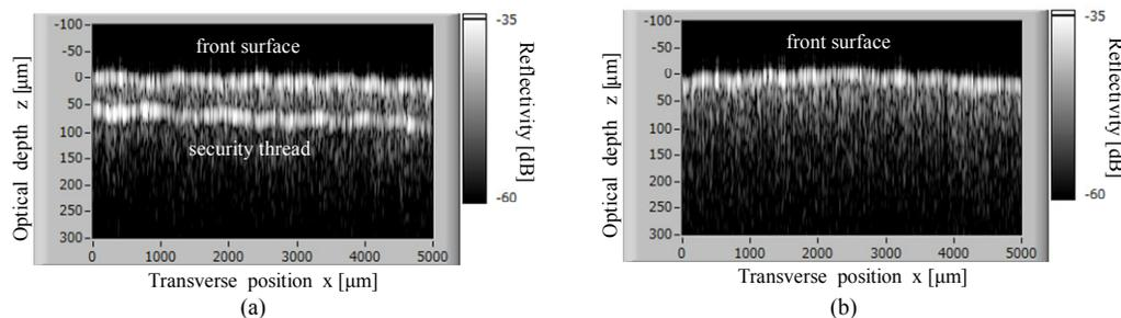
Fig. 4. Cross-sectional OCT images obtained at (a) the security thread region and (b) the no-security-thread region. Each image is composed of  $500 \times 400$  (transverse  $\times$  depth) pixels.
