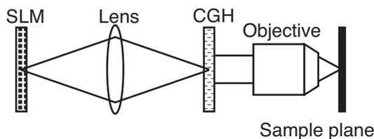
Fig. 1. A primal configuration of a hybrid diffractive system.
