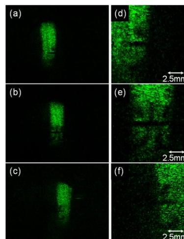
Fig. 4. Reconstructed images of the magnified light pulse. (a)-(c) Three scenes extracted from the obtained moving picture, (d)-(f) enlarged images of the light pulse shown in (a)-(c), respectively.
