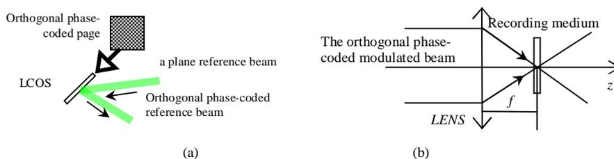
Fig.1 The scheme of building up of the orthogonal phase-coded beam (a), and the Fourier transform configuration for the reference beam (b).
