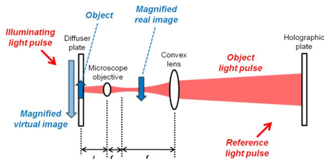
Fig. 2. Principle of the recording of the magnified image
