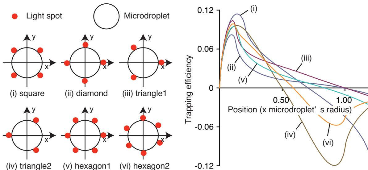
Fig. 2. The considered optical patterns consisting of multiple spots (left) and dependence of trapping efficiency on relative position (right).
