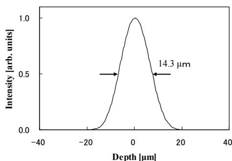
Fig. 3. Point spread function (PSF) measured using a mirror as a sample. FWHM axial resolution was estimated to be 14.3  $\mu\text{m}$  in air.
