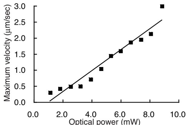
Fig. 4. Relationship between the maximum transport velocity and total illumination power.
