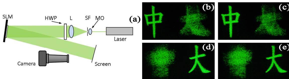
Fig. 1. (a) Set-up for optical reconstruction. MO: microscope objective, SF: spatial filter, L: lens, HWP: half-wave plates. Reconstruction in 800mm for (b) Fr-CGH and (c) Fh-CGH; in 1100mm for (d) Fr-CGH and (e) Fh-CGH.
