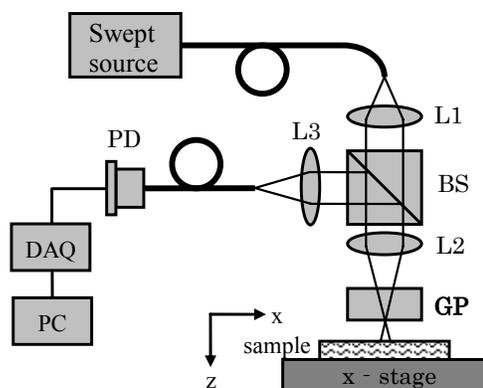
Fig. 1. Experimental setup of the common-path SS-OCT.
