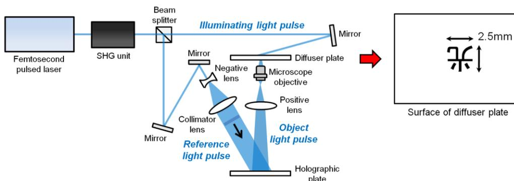
Fig. 3. Schematic diagram of the optical setup in the experiment
