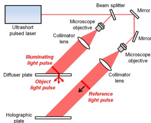
Fig. 1. Basic recording arrangement of LIF holography
