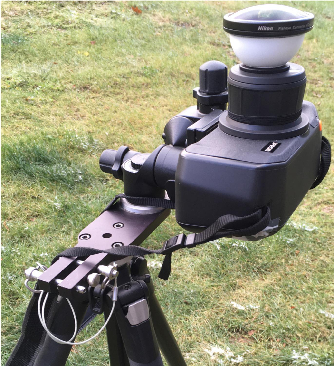
To acquire such all-sky spectra, use another hyperspectral camera: a Specim IQ imaging spectrometer fitted with a Nikon FC-E8 fisheye.
