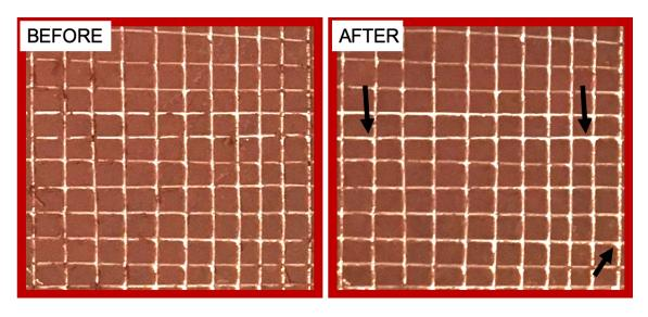
Cross-hatch test ASTM D3359-Method B
